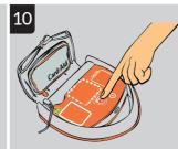
If electroshock is required, CardiAid informs the user and prepares the shock automatically. In CTO207RS, electroshock is delivered by pressing the button. In CTO207RF, the device delivers the shock automatically after warning the user
