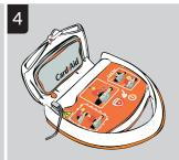
CardiAid switches on automatically when the cover of the device is opened. Follow the verbal and visual instructions
